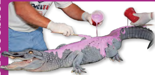
FastCat™ 30 is used with Mold Max™ 30 to make a mold of this frozen alligator.
